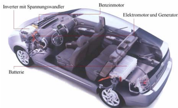
Abb. 2: Systemaufbau Toyota Prius (Toyota Hybrid-Synergy-Drive®)
